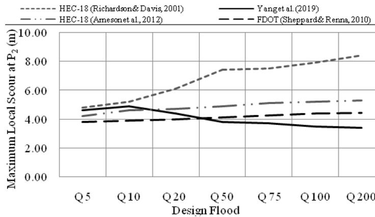
Figure 8: Local scour predicted using four empirical equations
