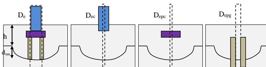
**Figure 2: A conceptual explanation of how to calculate  $D_e$  using the total of the individual diameters of each pile-supported component; the column, pile cap and pile group is provided. While factor  $h$  represents approaching water depth,  $d_{sm}$  represents the maximum local scour depth (Motivated by Moran)<sup>47</sup>.**
