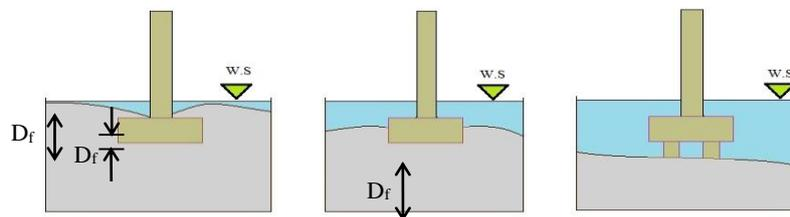
**Figure 3: Description of the height of foundation ( $D_F$ ) based on the alluvial riverbed levels from (a) to (c); surface water is denoted by W. S.**
